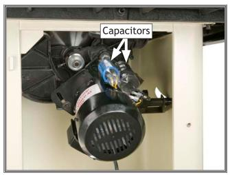
Figure 110. Motor capacitor location.
